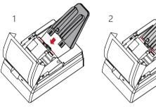
Please be sure the film feeder is inserted properly and secure before proceeding.
